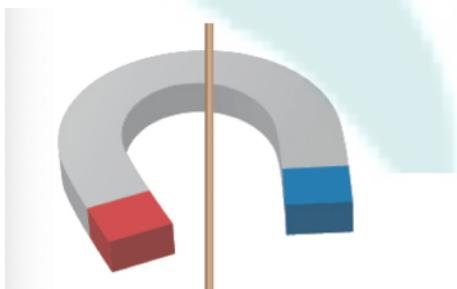
4. A length of flexible, slack copper wire is fixed so that part of it is held vertically in the field of a horseshoe magnet
